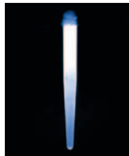
Light translucency of RelyX™ Fiber Post (size #2) here with the Elipar™ FreeLight 2 LED Curing Light. Source: 3M ESPE internal data
