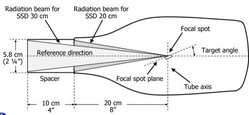
Note. The position of the focal spot is marked on the outside of the tube-head with a dot embossed on the top and bottom covers.
