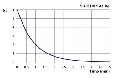
Tube Head Cooling curve
