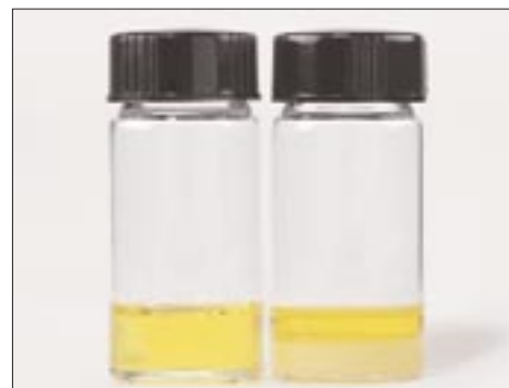
Figure 3. (l) Nanofiller in Adper™ Single Bond Plus Adhesive remains in solution; (r) filler in Optibond Solo Plus™ does not.
